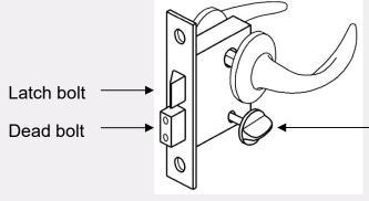
Note. The 'thumb-turn' operated lock should be sited on the room side of the door to facilitate escape without the use of a key.
